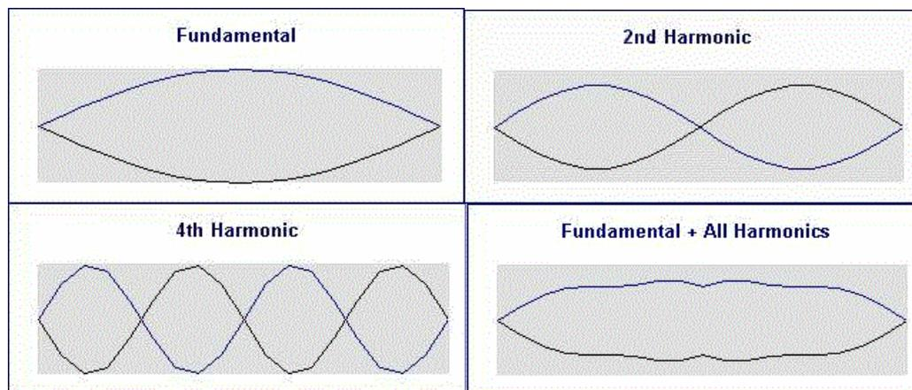
The single coil strat neck pickup reads the string at a single point exactly  $1/4$  the length of the string from the bridge (where the 24th fret would be), although some more recent 22-fret strats have the pickup a fraction towards the bridge.
