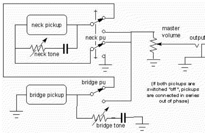
The next schematic gives a useful arrangement for 2 humbucking pickups incorporating coil taps and phase switching. There are a couple of special features in this circuit. Changing to "out of phase" while in the single coil mode changes the coil used in the bridge pickup, offering another sound while using just the bridge pickup.
